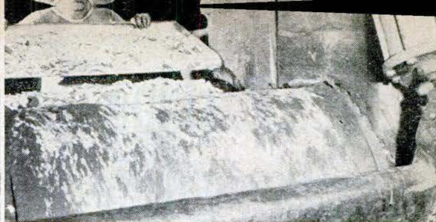
2 MARBLEIZING begins at the sheeting mill. Here an operator adds pigment chips (a modified tile mix) to doughy mass that came out of the Banbury. When it is now fed between rollers, the chips are distributed throughout. Plain-colored tile is also made.
